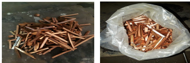
Figure1.2: Copper billets cut into small pieces
