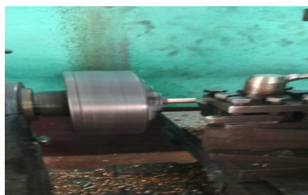
Figure:1.8 Machining of Casted Product
