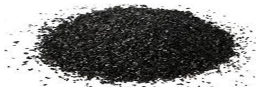
Fig 1. Granular Activated Carbon
