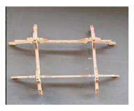
The skeleton of the drone which all componentry is fixed to. The frame design is a trade-off between strength (especially when additional weights such as cameras are attached) and additional weight, which will require longer propellers and stronger motors to lift
