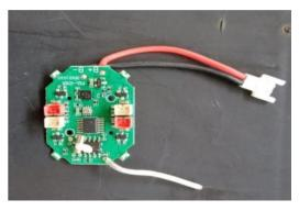
A controller is a circuit board that manages the drone's flight. Put simply, the flight controller's job is to control the power, or RPM (Revolutions Per Minute), for each individual motor on the drone in response to the information received from the drone controller.
