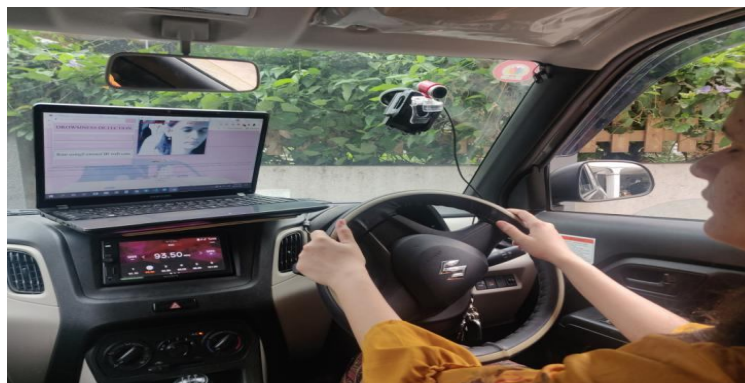
Fig 4.3: Drowsiness Detection using External Webcam.
