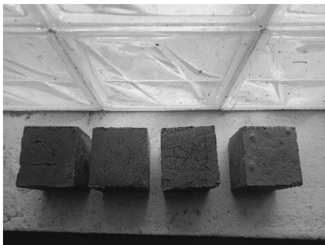
Fig. 1: 75mm cubes of different molarity
