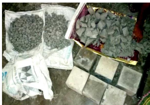
Fig. 2: Formation of geopolymer Coarse aggregate
