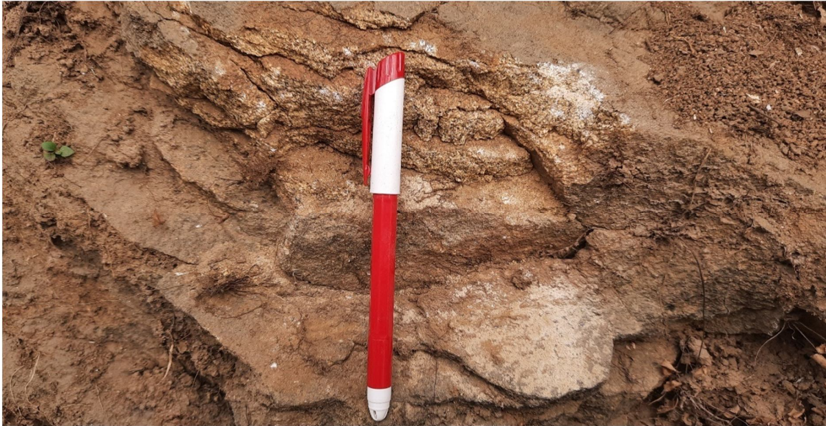
Fig. 2 Field photograph showing weathered granitic rock of Location 1
