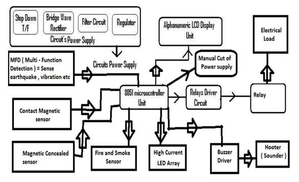
In this diagram, various blocks present the working of circuit.
