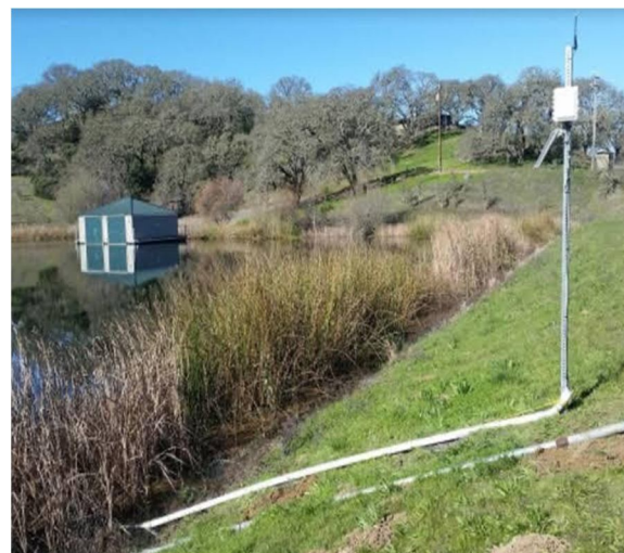
Actual Image of Water level Sensor.
