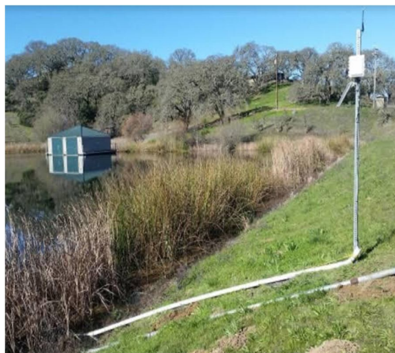
Actual Image of Water level Sensor.
