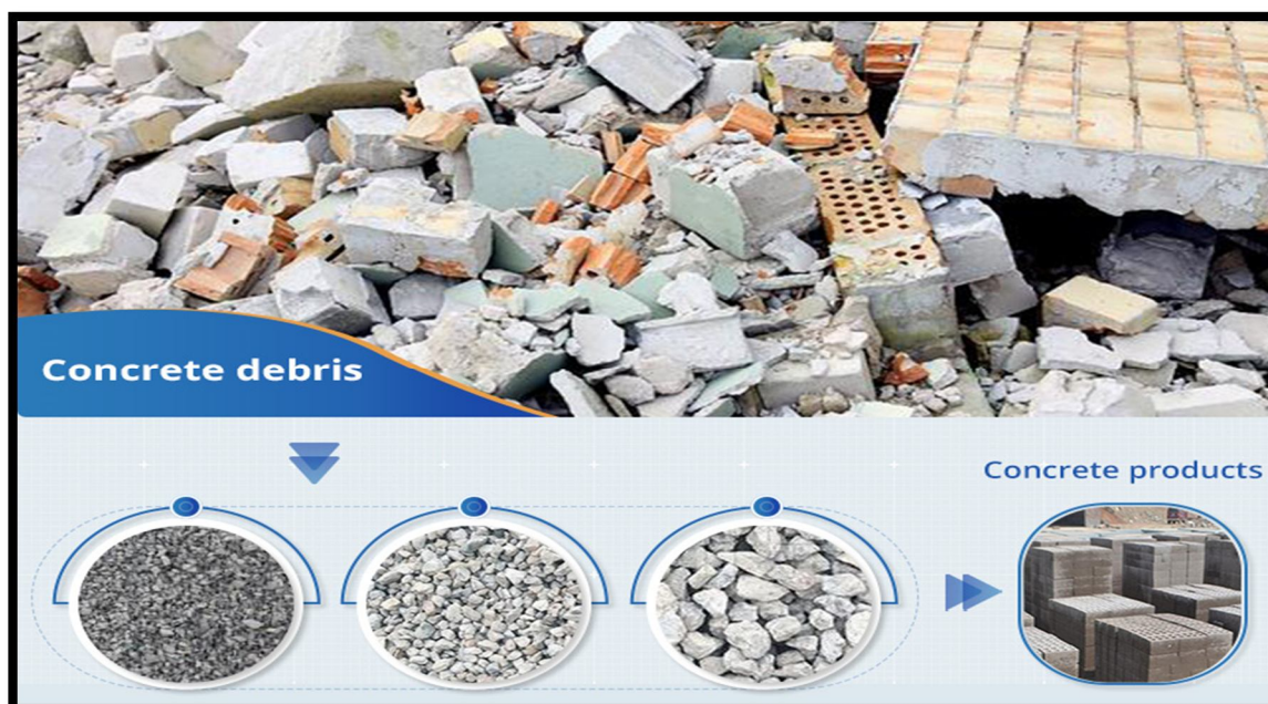
Figure: Production Of Concrete Blocks From Recycled Aggregate Concrete
