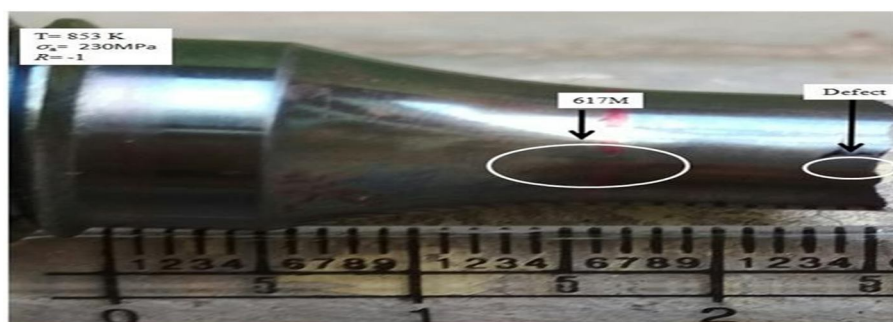
Fig.4.13: Failure location of DDMW HCF tested sample at 853 K, \sigma_a = 230 MPa, R = -1 .
