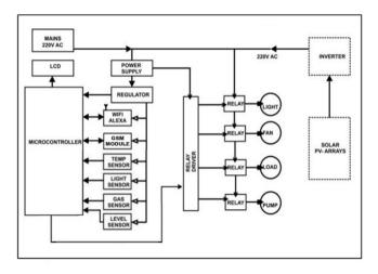
Block diagram, shows that solar arrays are used for the generation of electrical energy. DC power it connected to the inverter to convert AC power . the output of the inverter is 220v50Hz. Which is connected to the stepdown transformer to convert 220v into 12v. microcontroller gives the output command to the relay drive and relay turn on/off the load application from the recived command from the microcontroller.
