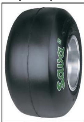
Fig. 3. Typical go-kart slick tire.
