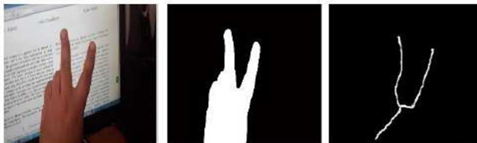
Fig. 2 Image background subtraction and erosion
