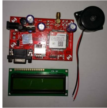
Fig.2 GSM modem with LCD display and Buzzer
