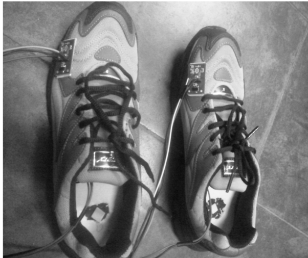
Fig. 4 Sensors Attached to the Shoes
