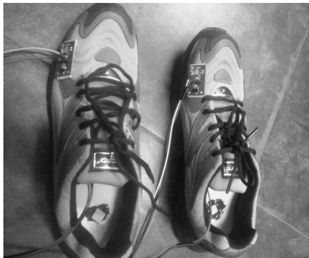
Fig. 4 Sensors Attached to the Shoes
