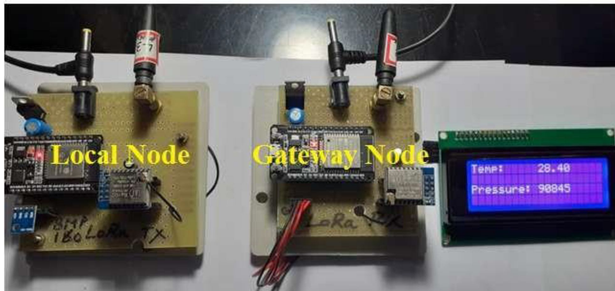
Fig. 3 Experimental setup with results on LCD display
