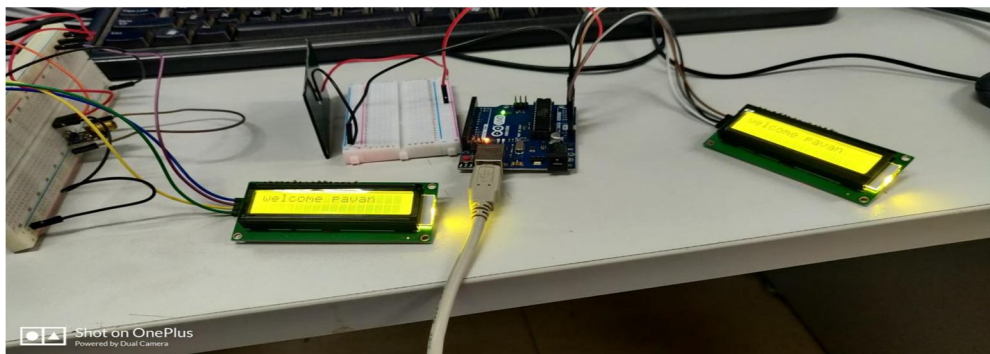
Fig 7: After we have added the lcd's the data is displayed at both ends i.e at the sender side after entering the data and receiver side after receiving the data it is shown as below
