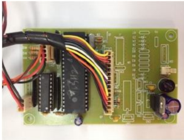
Fig. 7. PCB showing buffer, microcontroller and power supply
