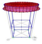
6) Circular Water Tank with Knee Bracing
