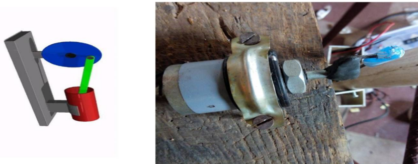
Fig-4. Blockage removing system
