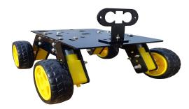
This is a vehicle on which the whole system is placed and moves throughout the field. The wheels are connected to two DC motor for the movement of the vehicle and the whole system is on the vehicle which moves around the field for ploughing and seeding.
