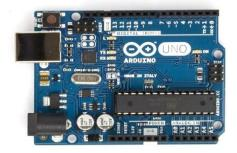
Arduino uno is a device with a microcontroller named atmega328p. This includes analog pins, digital pins and PWM pins. This is used to control the whole system according to the code given to it. The arduino is connected to rectifier and regulator. This microcontroller processes the internal program. This microcontroller is the heart of the project.
