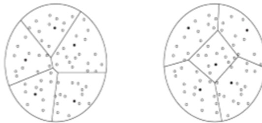
Figure 3: Adaptive clustering of the network. (• indicates Cluster Head )
