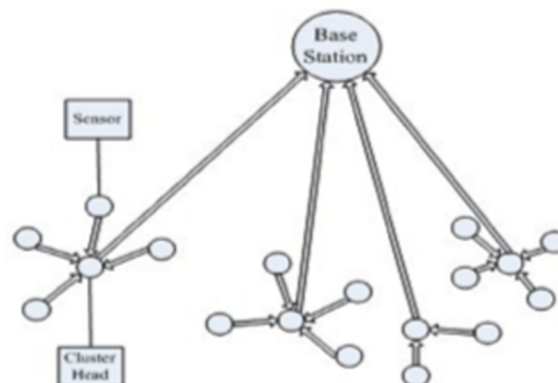
Figure 4: WSN Architecture for LEACH
