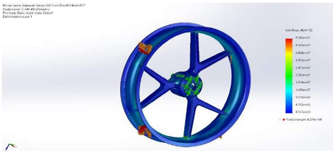
Fig c.1 Ti-6Al-4V static nodal stress-stress1
