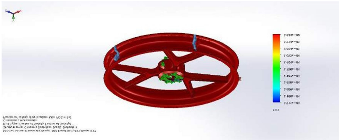
Fig b.4 Chrome Stainless Steel-Factor of Safety-Factor of Safety1
