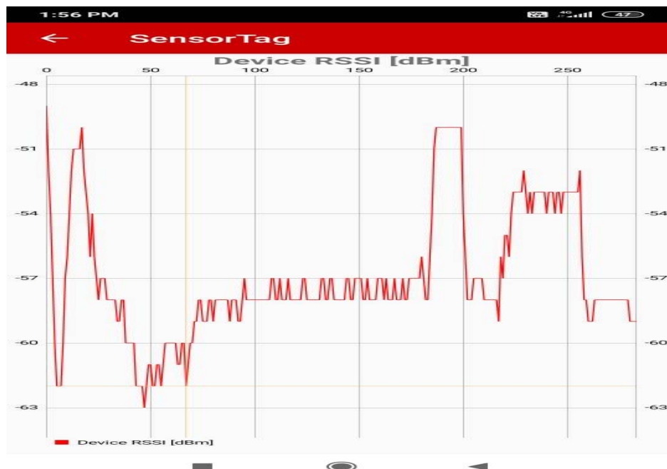
Fig 7 : : RSSI vs sampling-time graph of Bluetooth Low Energy obtained by TI SensorTag.
