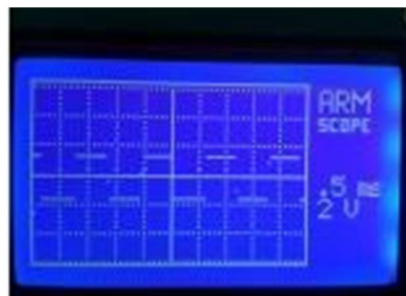
Figure 6.2: 3V and 1KHz Square Wave
