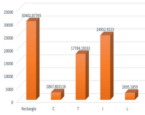
Fig:11 Storey shear Y Direction.
