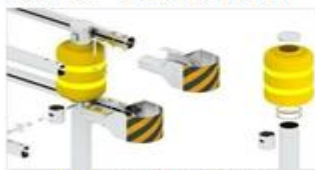
Joint system of rolling barrier
