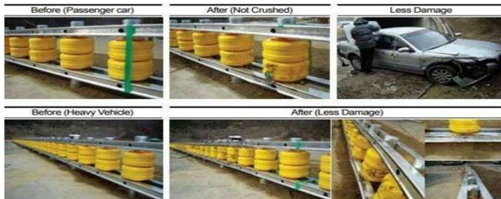
Figure.4.2.2. Crash test for car and truck collision at RB (KSI Korea)
