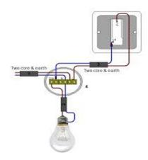
A one way lighting circuit is a simple circuit that enables one circuit to be turned on or off with one switch. The single circuit may have one or more lights in it. This type of circuit uses a one way switch. A wiring diagram is shown to the right, and a circuit diagram below.
