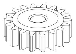
They consist of a cylinder or disk with teeth projecting radially. Though the teeth are not straight-sided but usually of special form to achieve a constant drive ratio, mainly involute but less commonly cycloidal, the edge of each tooth is straight and aligned parallel to the axis of rotation. These gears mesh together correctly only if fitted to parallel shafts. No axial thrust is created by the tooth loads. Spur gears are excellent at moderate speeds but tend to be noisy at high speeds.
