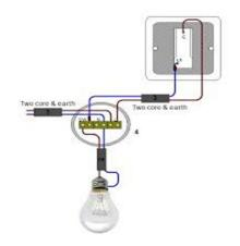
A one way lighting circuit is a simple circuit that enables one circuit to be turned on or off with one switch. The single circuit may have one or more lights in it. This type of circuit uses a one way switch. A wiring diagram is shown to the right, and a circuit diagram below.
