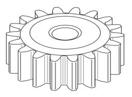
They consist of a cylinder or disk with teeth projecting radially. Though the teeth are not straight-sided but usually of special form to achieve a constant drive ratio, mainly involute but less commonly cycloidal, the edge of each tooth is straight and aligned parallel to the axis of rotation. These gears mesh together correctly only if fitted to parallel shafts. No axial thrust is created by the tooth loads. Spur gears are excellent at moderate speeds but tend to be noisy at high speeds.
