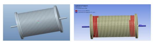
The rope drum should be made of seamless pipe machined & grooved accurately, to -ensureproper seating of wire rope in a proper layer. The drum should be fitted with two heavy duty Ball Roller bearings of reputed make for smooth operation & longer life. Drum length =pitch x ground height x no of rope fall/drum dia =35x10000x8/667 =4197mm [let ground height be 10m] Average drum thickness = h+h/2 = 31.9+7.1/2 =35
