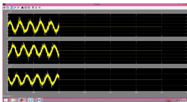
Figure 4: Waveform of three-phase fault voltage.
