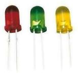
LED stands for light emitting diode. It is a semiconductor light source which emits light because of the flow of current through it .that is because of the combining of the electron and electron hole. Which releases energy in the form of photons.
