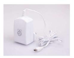
The supply of power differs from Pi model to model. Generally 5.1V is the supply which required to all the model but currently the supply is increasing according to the model. Raspberry Pi 4 uses a USB-C connector. While all other model up to Raspberry Pi 3 require a micro USB power connector.
