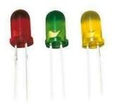
LED stands for light emitting diode. It is a semiconductor light source which emits light because of the flow of current through it .that is because of the combining of the electron and electron hole. Which releases energy in the form of photons.
