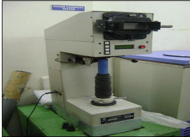
Figure 5.8 Vickers hardness test in urja laboratories.
