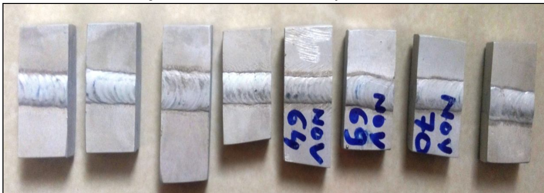
Figure 5.9 Vickers hardness Test Specimen As Per (IS:1500-2005)
