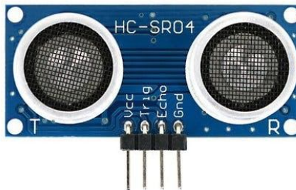
Fig. 9 Ultrasonic sensor HC-SR04
