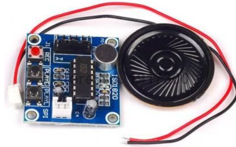
Fig. 11 ISD 1820 Voice recording module
