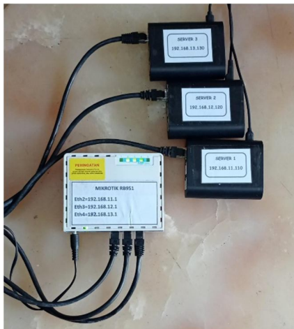
Fig. 2 VoIP Server with Raspberry Pi 3
