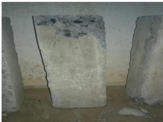
Figure 4 : Virgin specimen after testing
