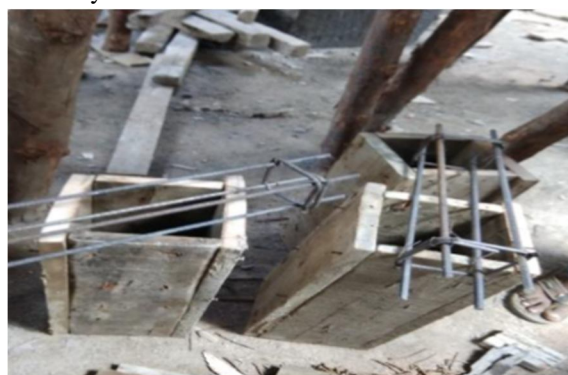
Figure 2: Mould & Reinforcement for virgin Specimen
