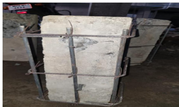
Figure 5: Virgin specimen with concrete jacket
