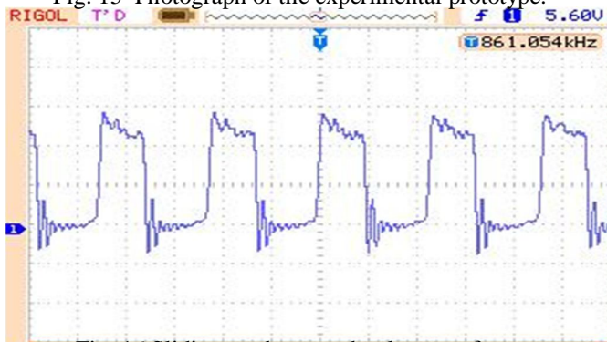
Fig. 16 Sliding mode control pulse waveform.
