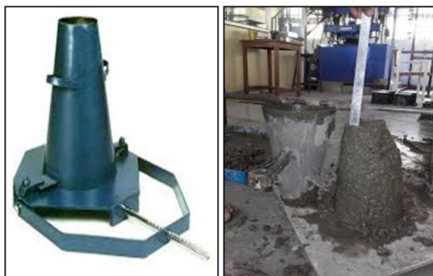
Fig. 6 Slump Cone Test for Workability
