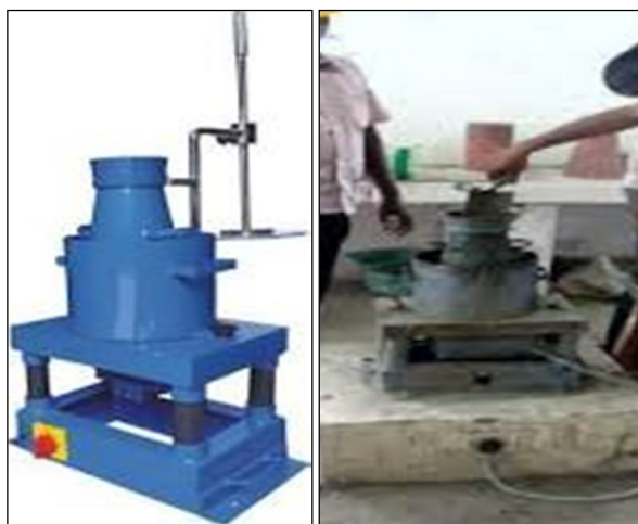
Fig. 8 Vee-Bee Consistometer Test for Workability
