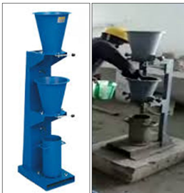
Fig. 7 Compaction Factor Test for Workability
