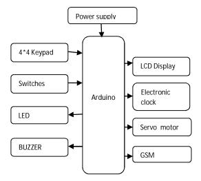
LCD 2084, Buzzer and GSM module is a yield gadgets which runs on the contribution of ATmegha16 microcontroller.
