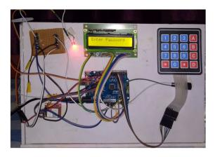
Present time will be saved in RTC module and notification time will be saved in EEPROM. Therefore at the time of taking medicines system generates notification sound and led starts to blink. Then the patient needs to apply correct password and take out the medicine and he/she should turn off the switch so that message will not send to the caretaker if the patient fails to do so then the system sends message to the caretaker.
