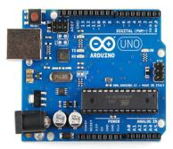
It's anything but an open-source stage utilized for building hardware projects. Arduino comprises of both an actual programmable circuit board (frequently alluded to as a microcontroller) and a piece of programming, or IDE (Integrated Development Environment) that sudden spikes in demand for your PC, used to compose and transfer PC code to the actual board Buzzer.
