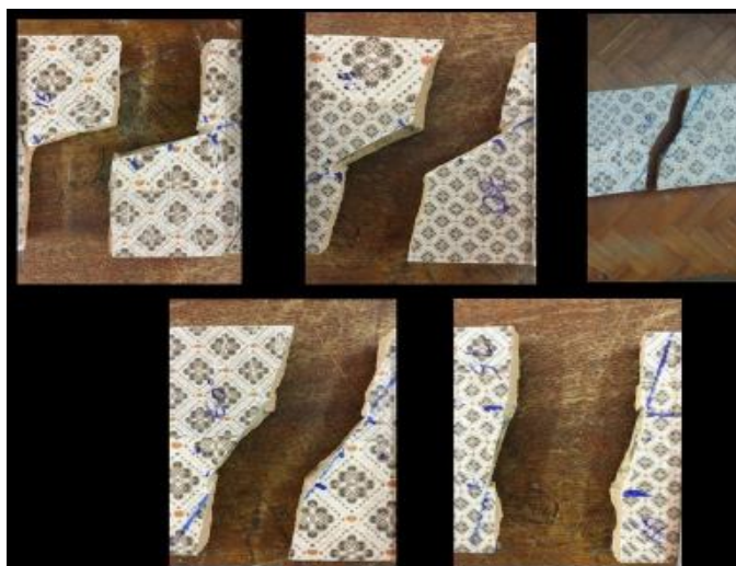
Fig. 3 Cracked brittle specimens with various inclination angle
