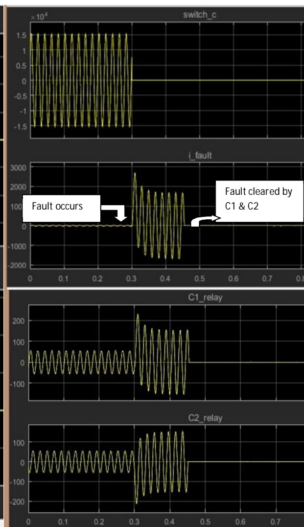
Fig. 8 simulation result when fault is cleared by backup protection provide by loop PDs.
