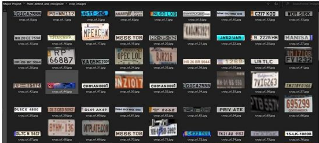
Fig. 3 Licence plates obtained from yolo model output
