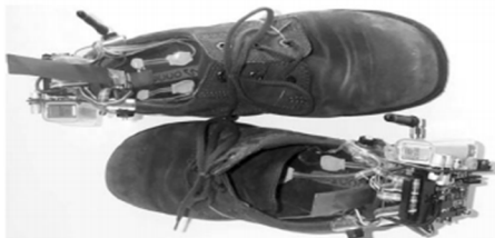
Figure 6. Shoe-integrated wireless sensor system, GaitShoe [5], showing all the hardware components.
