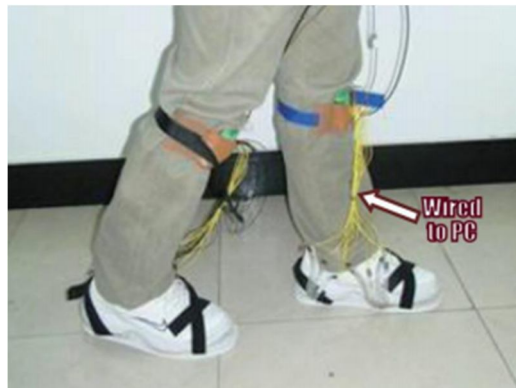
Figure 4. Identification based on dynamic plantar pressure in-shoe system [3].
