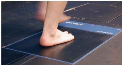
Figure 1. A platform-based foot planter pressure sensor emed® by Novel [1]
