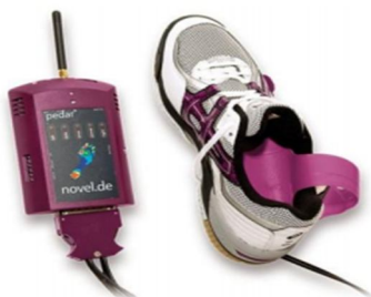
Figure 2. An in-shoe based foot planter pressure sensor by Pedar© Novel [1]
