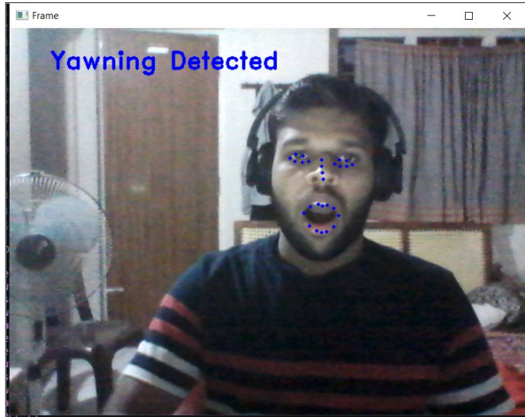
Fig. 5 Screenshot of warning message for yawning detection displayed on PC screen.
