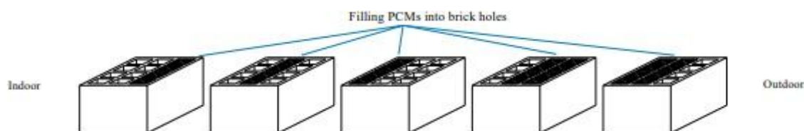
Fig 1. : Bricks filled with PCMs
