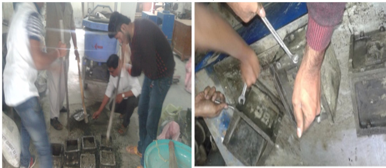
Fig. Preparation of Pervious Concrete Cubes
