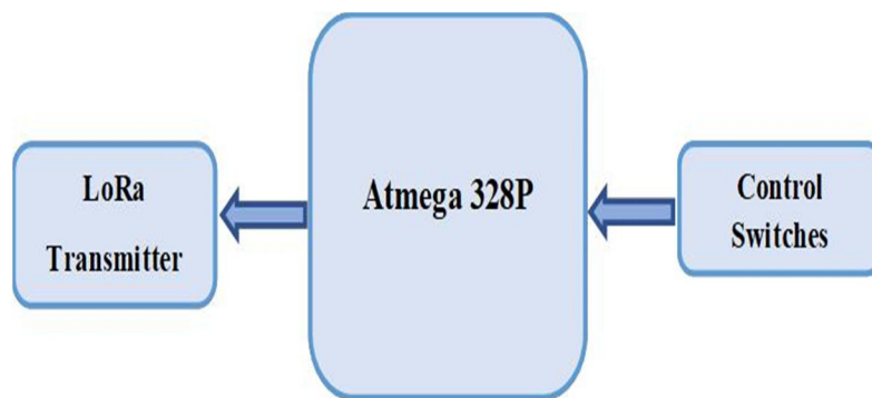
Fig. 1 Transmitter section block diagram
