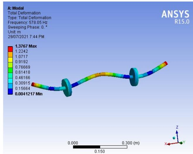
Figure No.12: sixth modes frequency of structural steel shaft
