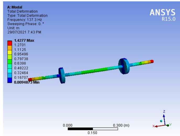
Figure No.8: Second modes frequency of structural steel shaft
