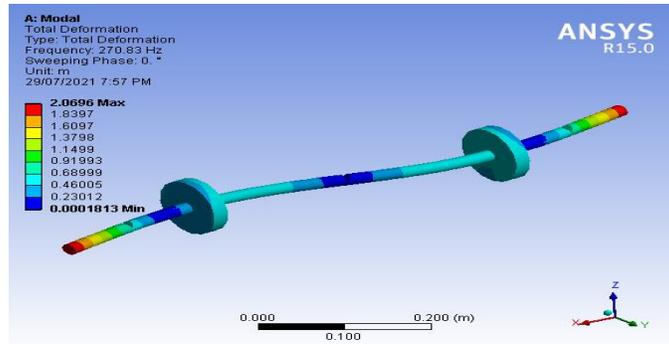
Figure No.16: fourth modes frequency of titanium alloy shaft
