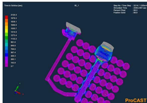
Fig.9 Total time to solidus with fraction solid
