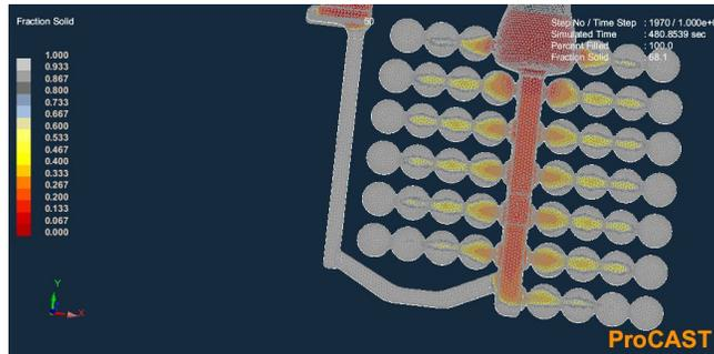
Fig. 10 Fraction solid of whole casting
