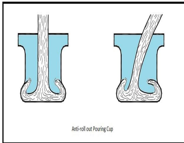
Fig. 2 Anti-roll pouring cups with metal fill-in
