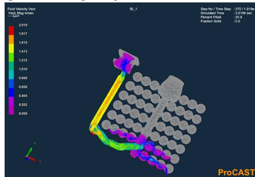
Fig. 11 Fluid velocity variation in the mould
