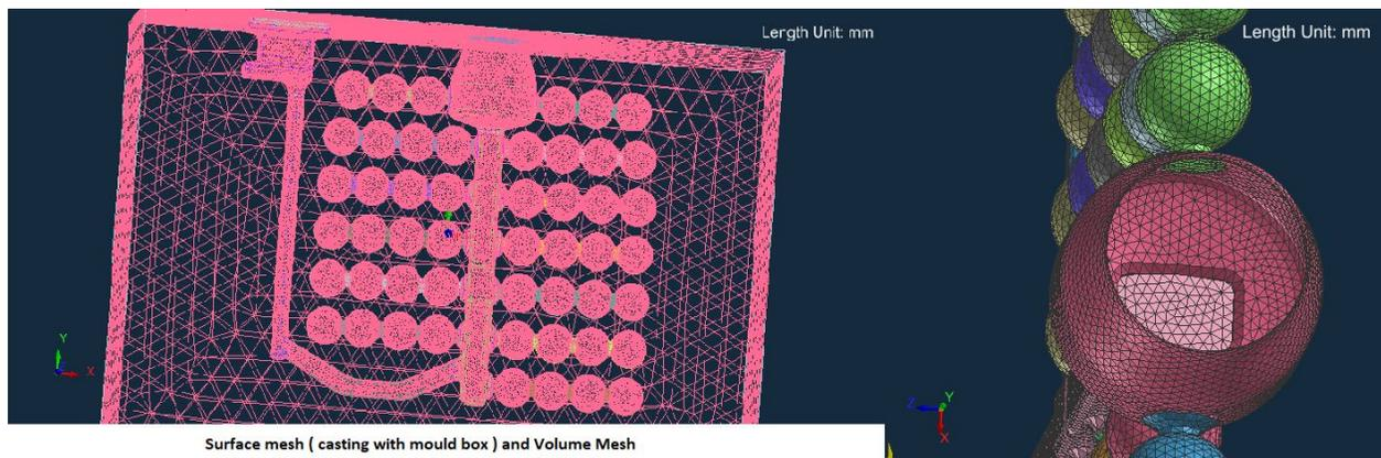
Fig. 5 Generated surface and volume mesh
