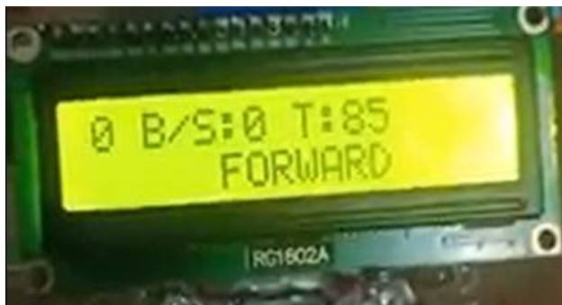
Fig. 4: Temperature sensor reading showing 85 degrees Celsius
