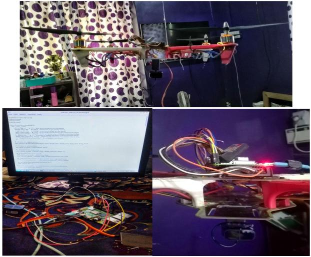
The Lidar module and servo motor are successfully interfaced with Raspberry-pi and all modules are successfully implemented on drone as shown in above figure and now drone is ready to fly.
