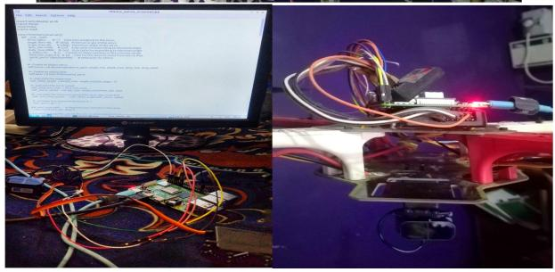
The Lidar module and servo motor are successfully interfaced with Raspberry-pi and all modules are successfully implemented on drone as shown in above figure and now drone is ready to fly.
